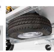
Spare wheel carrier for towing vehicle
